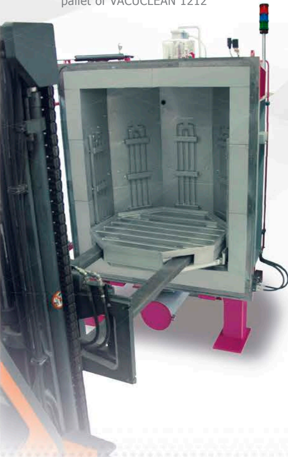
Process chamber and loading pallet of VACUCLEAN 1212
