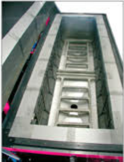
Process chamber of VACUCLEAN 254
