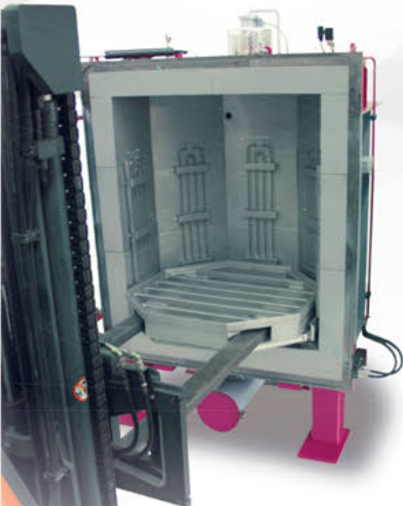
Process chamber and loading pallet of VACUCLEAN 1212
