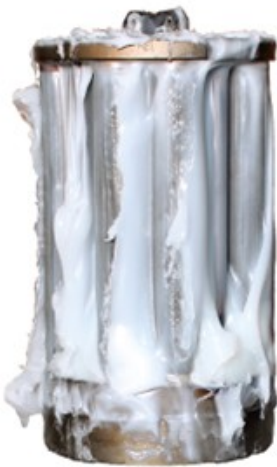
Photo: Filter bundles before cleaning
