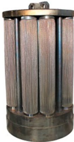
Photo: Filter bundles after cleaning
