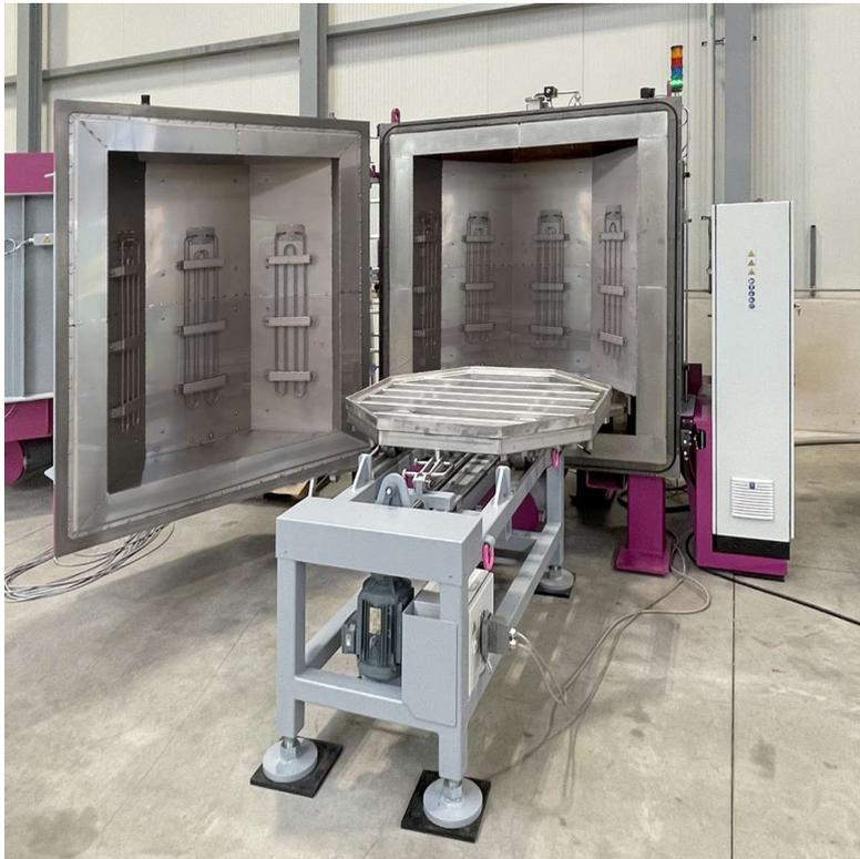
At the push of a button, the electrically driven loading pallet of the VACUCLEAN vacuum pyrolysis cleaning system can be moved forward or backward. The automation protects the cost-intensive tools and equipment, relieves the employees and requires less space, e.g. for maneuvering areas of forklifts
